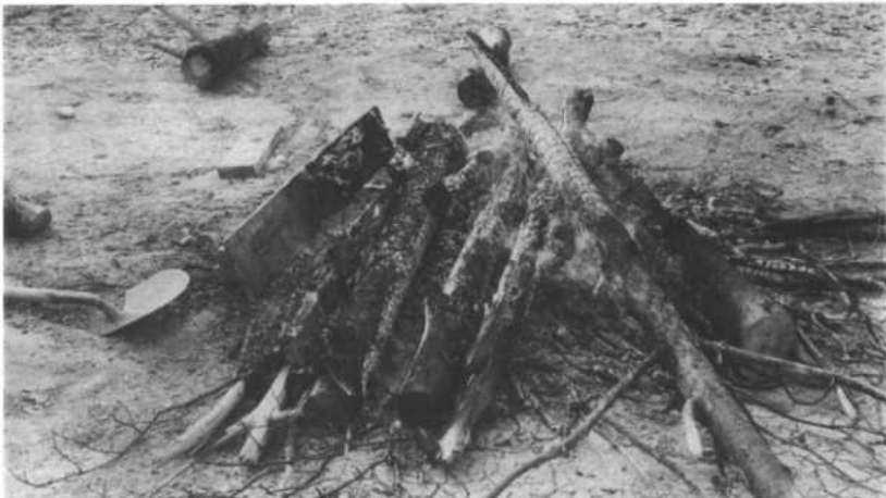
Fig. 7.3. Heat radiation had ignited the flaming half of the board on the ground, while the half near the shovel-painted white with a thick coating of slaked lime-had not even begun to smoke.
