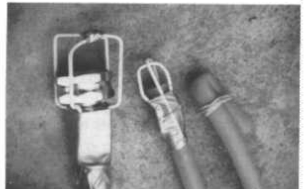
Fig. 8.8. Two wire "protectors," each made of two pieces of coathanger wire taped to a 1/2 inch flexible hose and a rubber tube. Shown on the right is a tube closed with a rubber band to stop a siphoned flow of water. (Illustration)
